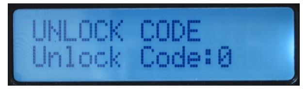
To unlock the device rotate the Volume/ Setup knob until the number 45 is displayed on the screen and then push the Volume/ Setup knob.
