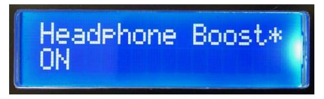
If 'ON' is not shown on the setup screen as per the above picture then headphone boost is turned off.
